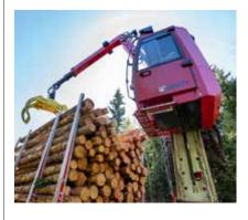
**High Seat** offers both standard mechanical crane controls and a cutting-edge electric joystick with an intuitive user interface that delivers smooth operation and precision. Featuring a refined safety system, High Seat is ergonomic, heated and weather-resistant, and it's easy to position since its fully adjustable.
